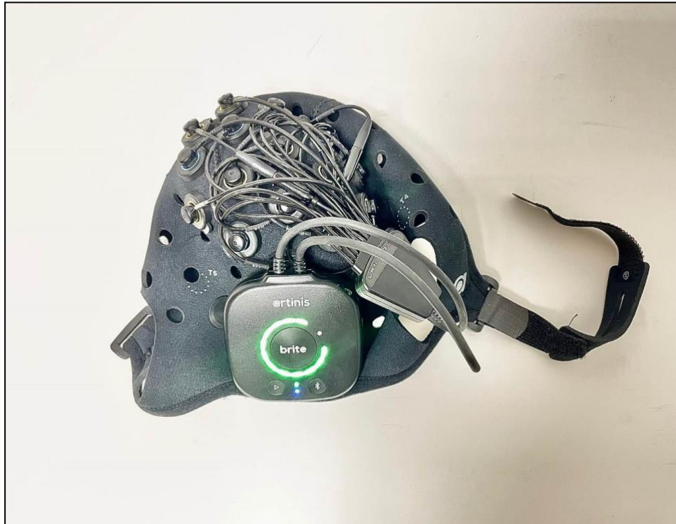
Figure 5. 27-ch fNIRS Artinis Brite wearable device
